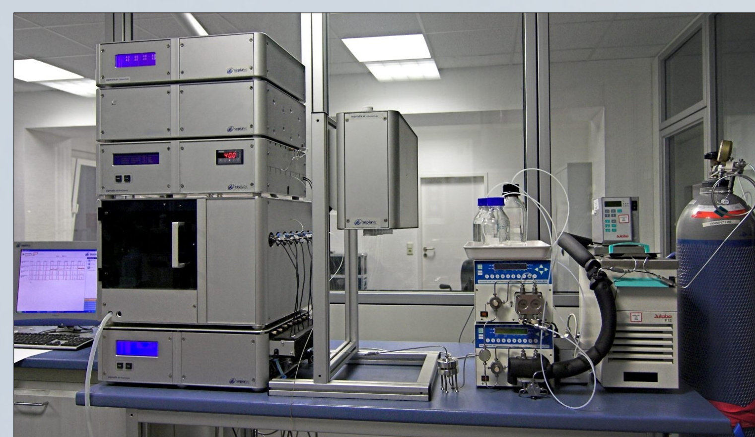
Fig. 4: Sepmatix 8x parallel SFC screening system (pre-series)
